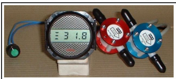
Bild 1) Red Cube FT-60 Flow Transducer
